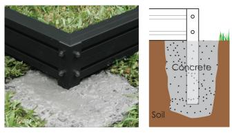
Corner stakes concreted into position requires a little more work, but provides a stronger anchor & better peace of mind knowing it's solidly anchored.
