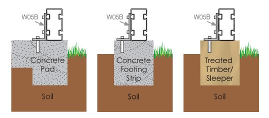
Attention: Double check your foundations are set level and square. Measure the diagonal lengths from corner to corner ensureing they are the same.
